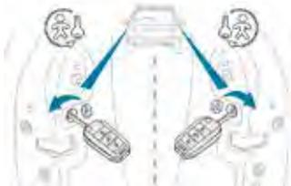
Mechanical system to prevent opening of a rear door using its interior control. The control is located on the edge of each rear door.
