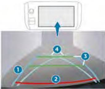
The blue lines **1** represent the general direction of the vehicle (the gap between these lines corresponds to the width of your vehicle including the mirrors).
