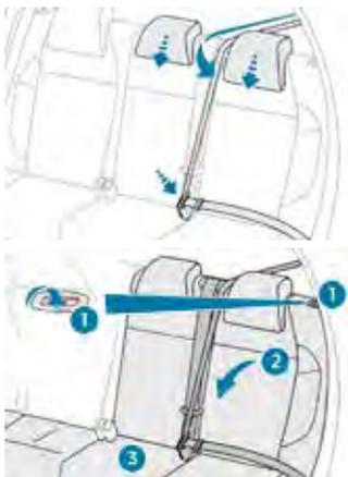
**!** When **returning the backrest to its initial position**, check that the seat belts are not trapped and that the red indicator at the control **1** is no longer visible.
