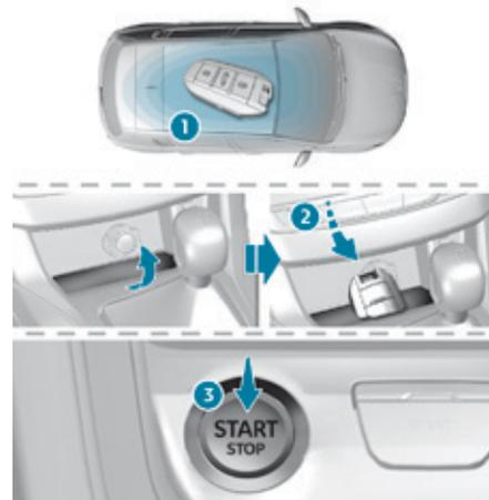
When the electronic key is in the recognition zone and your vehicle does not start after pressing the "START/STOP" button:
