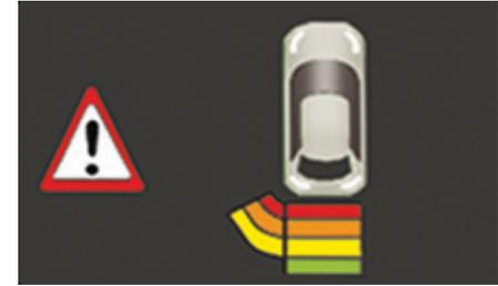
This supplements the audible signal by displaying bars in the screen or the instrument panel which move progressively nearer to the vehicle. When the obstacle is near, the "Danger" symbol is displayed.
