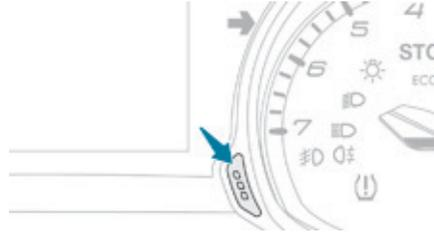
After each service, the service indicator must be reset to zero.
