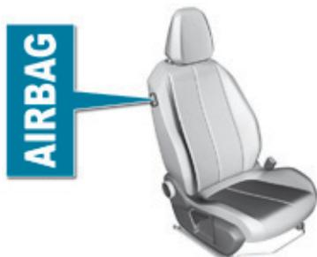
If fitted to your vehicle, this is a system which protects the driver and front passenger in the event of a serious side impact in order to limit the risk of injury to the chest, between the abdomen and head.
