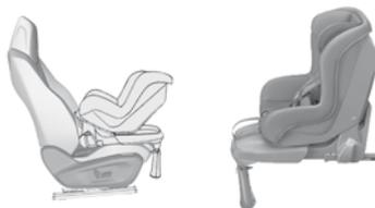
Installed rearward facing using an ISOFIX base which is attached to the rings **A**. The base has a support leg, adjustable for height, which sits on the vehicle's floor. This child seat can also be used forward facing. This seat can **not** be secured with a seat belt. We recommend that you use the seat in the rearward facing position up to the age of 3 years.
