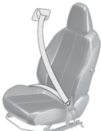
The front seat belts are fitted with a pretensioning and force limiting system. This system improves safety in the front seats in the event of a front or side impact. Depending on the severity of the impact, the pretensioning system instantly tightens the seat belts against the body of the occupants. The pretensioning seat belts are active when the ignition is on. The force limiter reduces the pressure of the seat belt on the chest of the occupant, so improving their protection.
