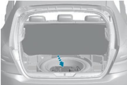
The tools are installed in the boot under the floor.
