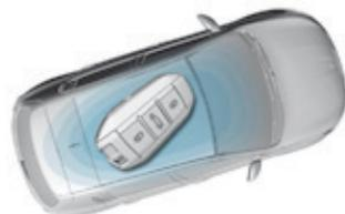
With the Keyless Entry and Starting remote control inside the vehicle, pressing the "START/STOP" button, **with no action on the pedals**, allows the ignition to be switched on. This also allows the accessories to be used (for example: audio system, lighting...).
