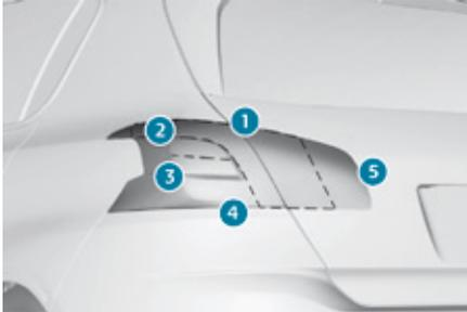
1. Sidelamps (light-emitting diodes - LEDs).
