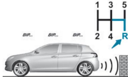
The proximity information is given by an intermittent audible signal, the frequency of which increases as the vehicle approaches the obstacle. The sound emitted by the speaker (right-hand or left-hand) indicates the side on which the obstacle is located. When the distance between the vehicle and the obstacle becomes less than approximately thirty centimetres, the audible signal becomes continuous.
