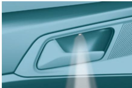
At night, the illumination of the interior opening controls on the front doors comes on automatically when the sidelamps are switched on.
