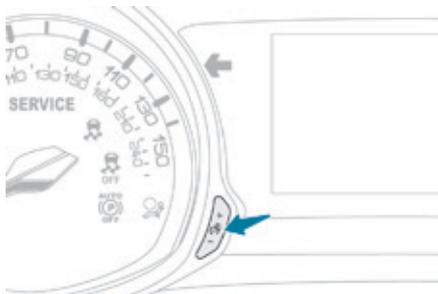
With the exterior lighting on, press this button to adjust the brightness of the dashboard lighting, the touch screen and the mood lighting. As soon as the lighting reaches the required level of brightness, release the button.
