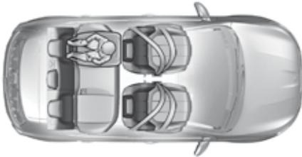
When a rearward facing child seat is installed **on a rear passenger seat**, move the vehicle's front seat forward and straighten the backrest so that the rearward facing child seat does not touch the vehicle's front seat.
