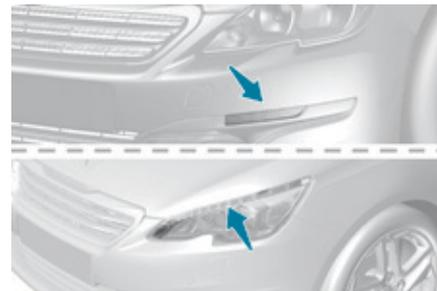
They come on automatically when the engine is started, when the lighting control stalk is in position **"0"** or **"AUTO"**.
