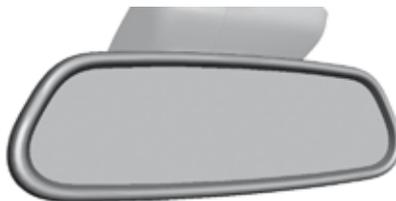
This system automatically and progressively changes between the day and night uses by means of a sensor, which measures the light from the rear of the vehicle.
