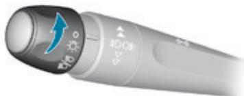
**O** Lighting off (ignition off) / Front daytime running lamps (engine running).
