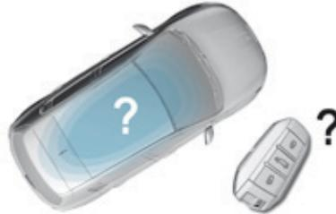
When the electronic key is not detected or is no longer in the recognition zone, a message appears in the instrument panel when you close a door or when you request switching off the engine.
