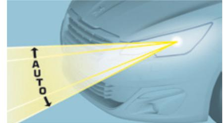
This system automatically adjusts the height of the beams from this type of headlamp, according to the load in the vehicle, to avoid causing a nuisance to other road users.
