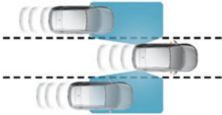
This driving assistance system warns the driver of the presence of another vehicle in the blind spot angle of their vehicle (areas hidden from the driver's field of vision), as soon as this presents a potential danger.
