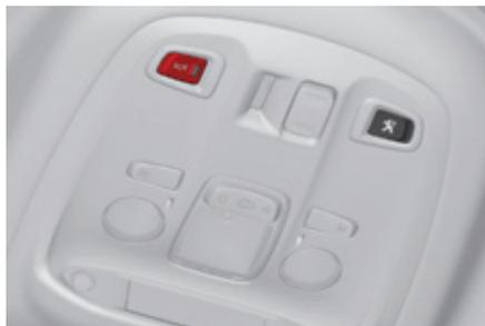
**!** If an impact is detected by the airbag control unit, and independently of the deployment of any airbags, an emergency call is made automatically.
