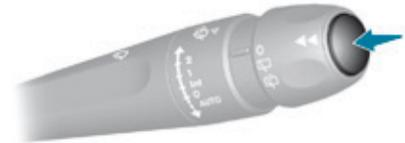
☞ Press the end of the wiper control stalk to display in the instrument panel the different information on dynamic settings.
