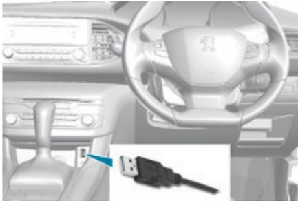
It allows the connection of a portable device, such as a digital audio player of the iPod® type or a USB memory stick.
