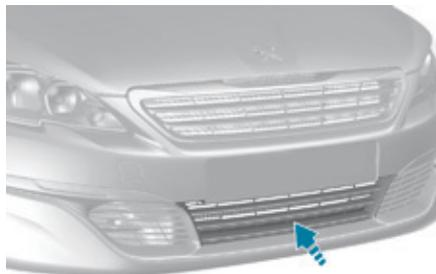
When towing, you must remove the blanking cover if your vehicle has one. Contact a PEUGEOT dealer or a qualified workshop for this.
