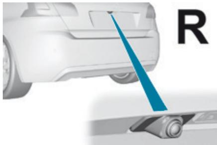
The reversing camera is activated automatically when reverse gear is engaged. Depending on version, the image is displayed in the touch screen or the instrument panel.
