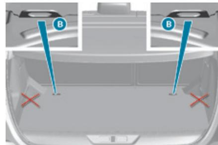
A ring **B** is located in the boot (indicated by a marking), referred to as the **TOP TETHER**, for fixing the upper strap.
