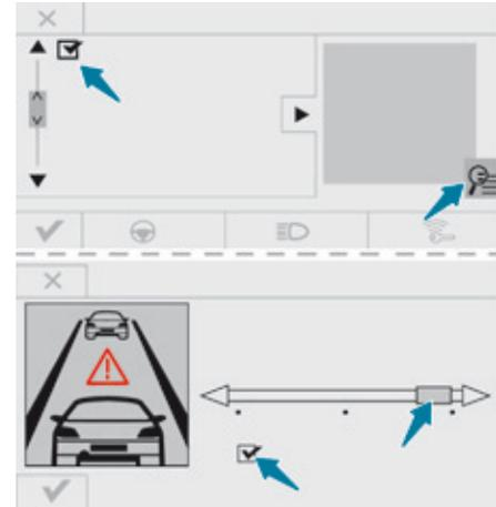
The emergency collision alert system can be activated or deactivated by the driver. From the secondary page of the "**Driving assistance**" menu:
