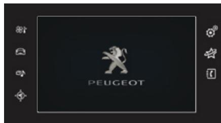
**i** In very hot conditions, the system may go into stand-by (screen and sound completely off) for a minimum period of 5 minutes.
