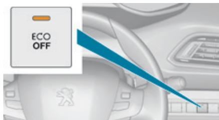
At any time, press the "**ECO OFF**" switch to deactivate the system. This is confirmed by the switch warning lamp coming on accompanied by a message.
