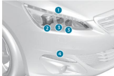
1. Daytime running lamps / sidelamps (light emitting diodes - LEDs).
