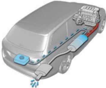
To assure respect for the environment and conformity with the new Euro 6 emissions standard, without adversely affecting the performance or fuel consumption of Diesel engines, PEUGEOT has taken the decision to equip its vehicles with an effective system that associates SCR (Selective Catalytic Reduction) with a particle filter (FAP) for the treatment of exhaust gases.
