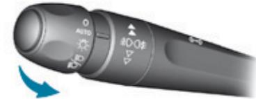
Temporarily keeping the dipped beam headlamps on after the vehicle's ignition has been switched off makes the driver's exit easier when the light is poor.
