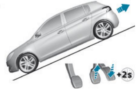
**On a descending slope, with the vehicle stationary and reverse gear engaged, the vehicle is held momentarily when you release the brake pedal.**
