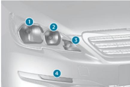
1. Dipped beam headlamps (H7-55W).
