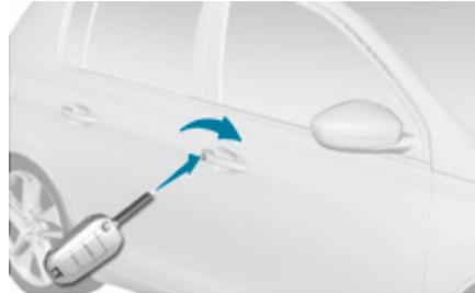
☞ Turn the key to the front of the vehicle to unlock the vehicle, then pull the handle to open the door.
