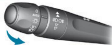
Pull the stalk to switch the lighting between dipped and main beam headlamps.
