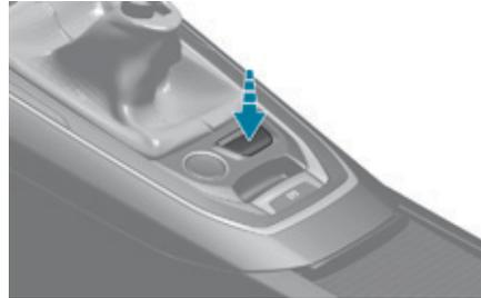
☞ Press and hold the button until the back-lighting in the instrument panel changes. The LED in the button stays on.
