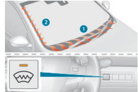
In area 1, the heating frees the wiper blades when they are stuck by snow or ice.
