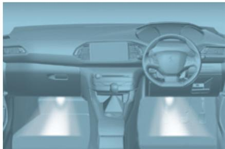
Its operation is identical to that of the courtesy lamps. The lamps come on when one of the doors is opened.
